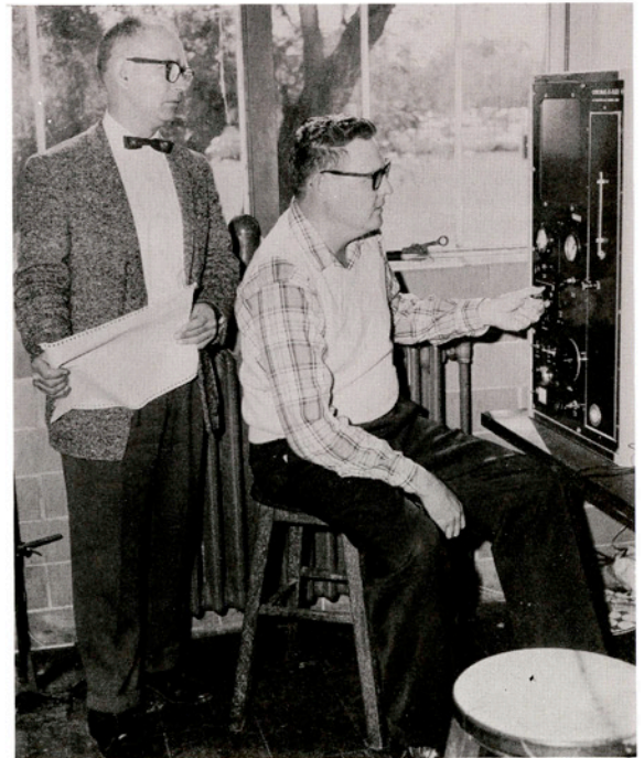
Dr. Fred Garland looks on as Dr. E. V. Ruhnke checks out the gas chromatograph.
