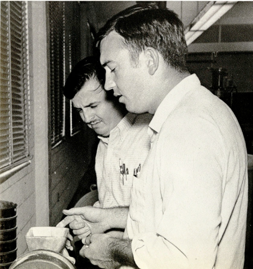
Joel Cavazos and Mike Riley place rocks through grinder in preparing samples for screen analysis in Engineering's Unit Operations Lab.
