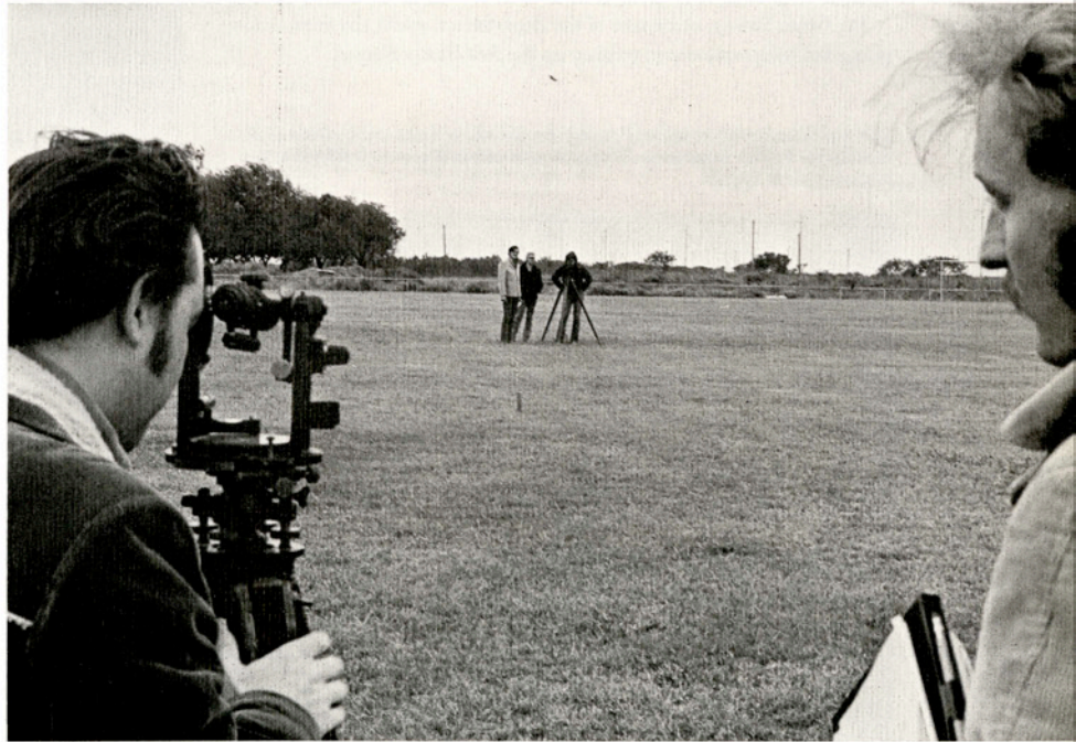
Top: An EE student from 457 class works with an analog computer which solves differential equations. Bottom: A survey class is practicing the use of a transit to measure the size of horizontal and vertical angles. Surveying is important in land ownership to know the correct configurations of boundaries and the area enclosed by boundaries.
