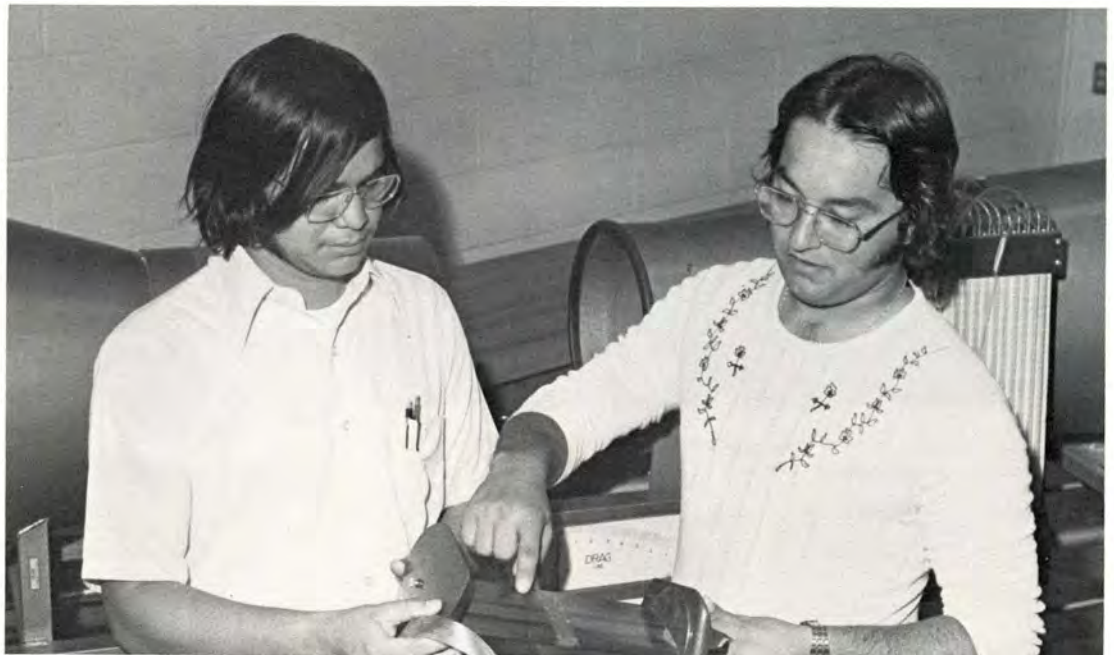
David Soliz and Alfredo Ramirez, III, both NASA scholarship winners, are measuring the lift and drag of an airplane wing in a wind tunnel.
